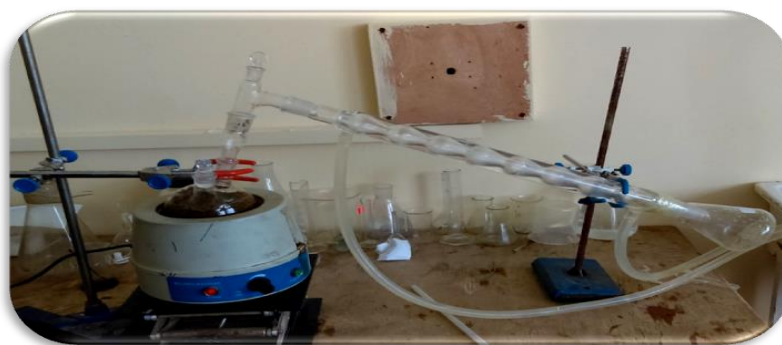
Fig. 2. Clevenger hydrodistillation setup.
