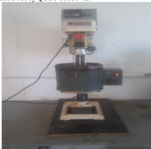
Figure 2. Mixer provided with heating
