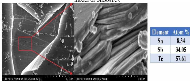
Fig. 4. Scanning electron micrographs of ingot composition with 75 mol% \text{Sb}_2\text{Te}_3 .
